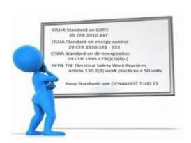
The OSHA standard for the Control of Hazardous Energy (lockout/tagout) is found in 29 CFR 1910.147. This standard addresses practices and procedures necessary to disable machinery and prevent the release of potentially hazardous energy while maintenance or servicing activities are performed.
