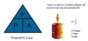
In this module we have discussed Pascal's Law and three primary factors that we can control in a hydraulic system: pressure, force, and area. We also discussed the hydraulic lever and the multiplication of force.
