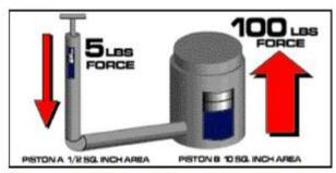
The difference in the areas of the two pistons determines the multiplication of force.
